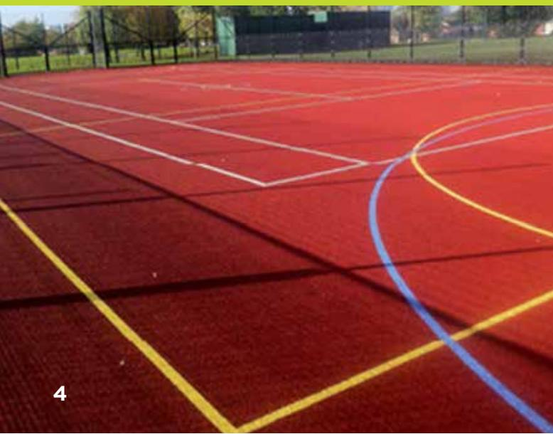
**Hard Tennis courts and multi use games areas (MUGAs) can be made of porous macadam (Tarmac). Without proper maintenance, moss, mould, leaf & stick debris and bird droppings contaminate the surface and eat into the macadam. This leads to the Tarmac breaking up, which makes holes and loose stone becomes present leading to a dangerous area.**
