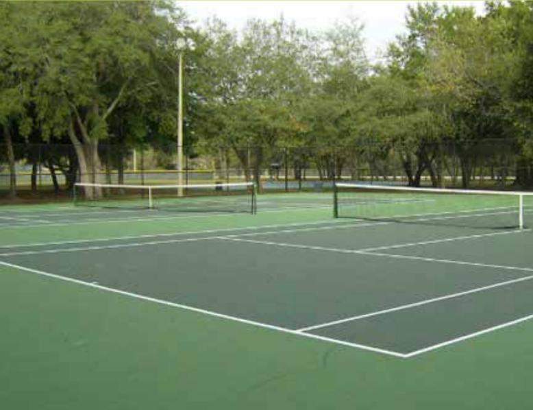
**The best of non-cushioned tennis surfaces, acrylic surfaces are prone to cracking and drainage issues due to the UK climate. A non-porous surface, which can sit in water for much of the year, it requires a good regular maintenance programme to ensure it does not become contaminated with mould, moss and algae.**
